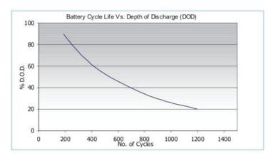
$\begin{array}{lll} \mbox{Nominal voltage} & 6 \& 12 \mbox{ volts} \\ \mbox{Design life} & 12 \mbox{ Years @ 20°C} \\ \mbox{Operating temperature} & -10 °C \mbox{ to } 45°C \end{array}$
